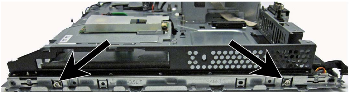
Figure 6-88 Display panel screw locations – 8300 models – CMI panel
